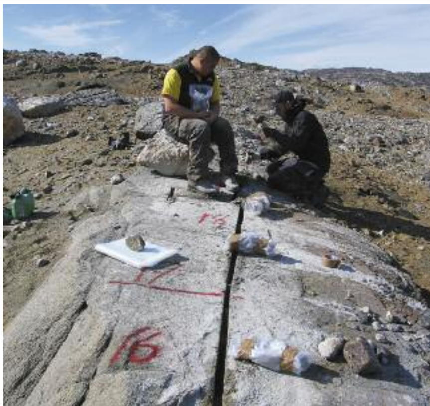
Detailed saw-channel sampling of the dunite-dominated ultramafic sills at Ikertoq in West Greenland. Photo: 21 st North.
