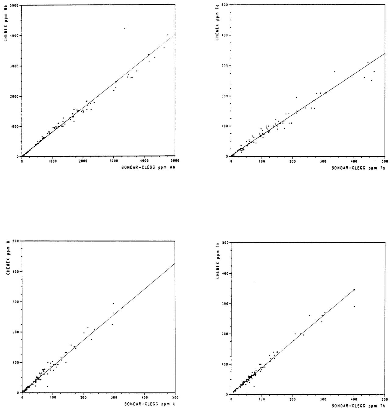
**Fig. 2.** Scatter plots of assay values from 92 chip samples analysed by two laboratories. The regression lines are calculated by the reduced major axis method.
