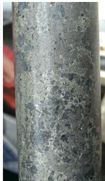
Massive sulphide sample from diamond drill hole MQ-13-026 at the Imiak Hill occurrence, part of the Maniitsoq Norite Belt. The sample, which comes from 158.5 metres down the hole assayed 5.26% Ni, 1.78% Cu and 0.18% Co. Photo: North American Nickel Inc.
