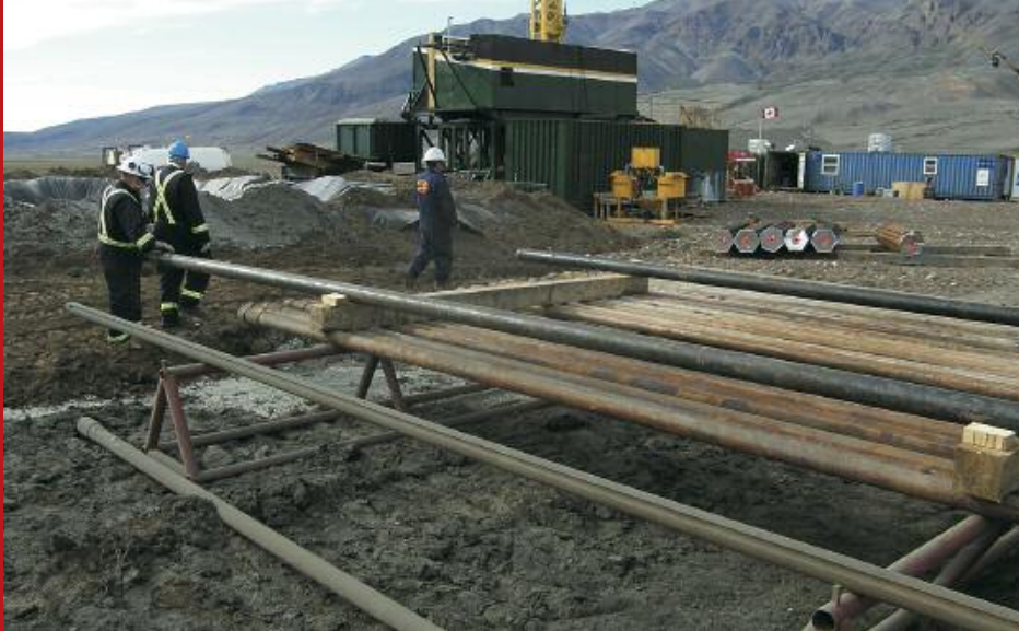
Drill rig and casings used in connection with Vismand Exploration Inc.'s drill programme on Nuussuaq in 2007. The aim was to locate nickel-enriched, deeper-lying, lava conduits that connect to successions of contaminated flood basalts.
