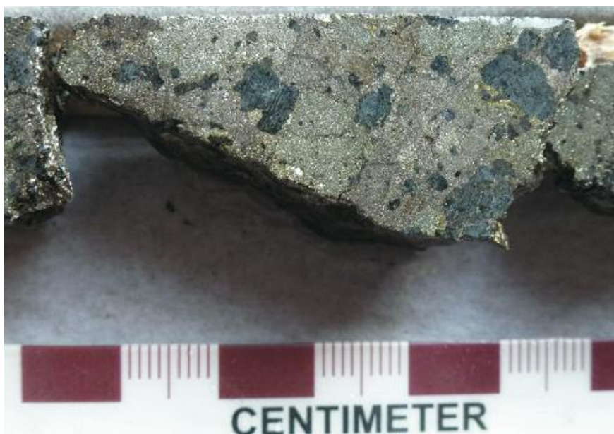
Coarse-grained pyrrhotite-pyrite-pentlandite-chalcopyrite mineralisation from Imiak Hill. Photo: North American Nickel Inc.
