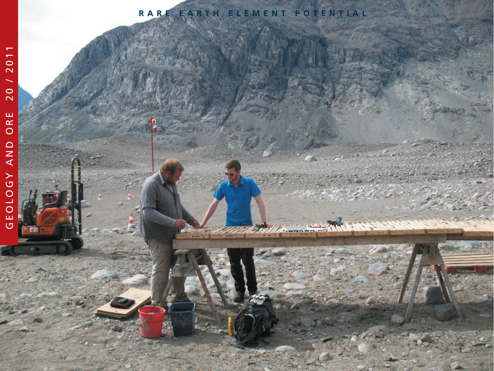
Drill core logging at the Motzfeldt Sø camp in 2011. Photo: Ram Resources Ltd.
