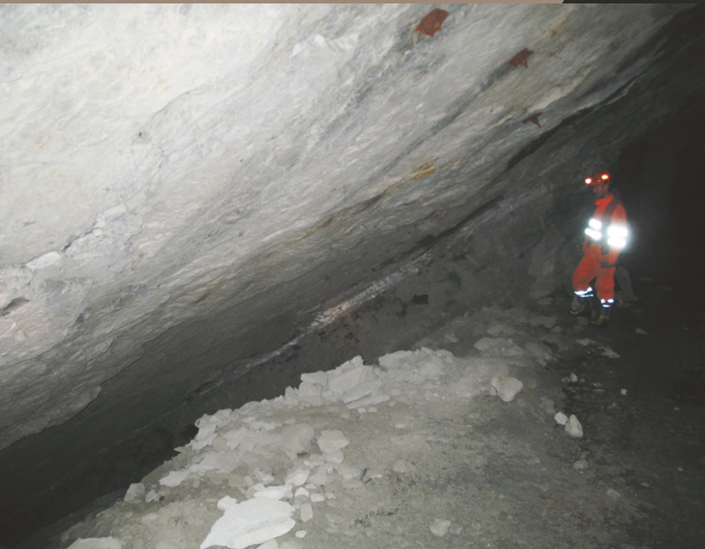
An underground view of a hanging wall of a mined-out 1.2 m stope.
