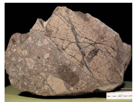
Cut surface of igneous breccia from the Flammefjeld complex. The large granitic fragment with stockwork molybdenum mineralisation runs 0.45% MoS 2 .
