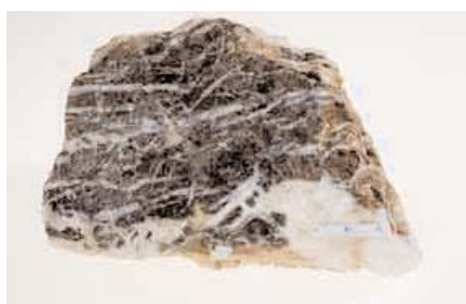
Typical lead and zinc ores from Blyklippen: Top: Grey galena and white quartz. Bottom: Brown sphalerite and white quartz. Sample length: 15 cm. Photo: GEUS.
