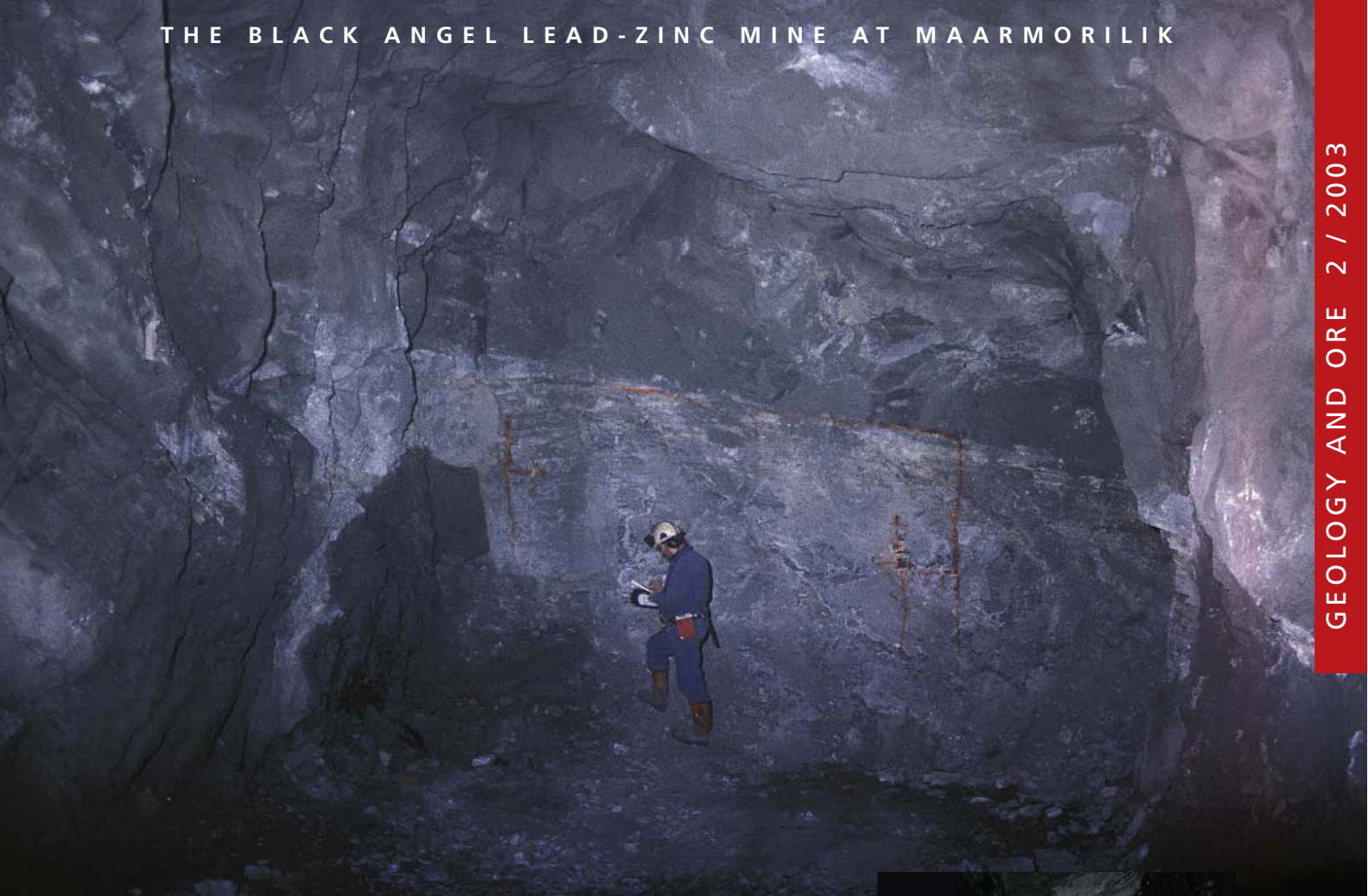
Typical face to be mined selectively: ore on top of white marble.
