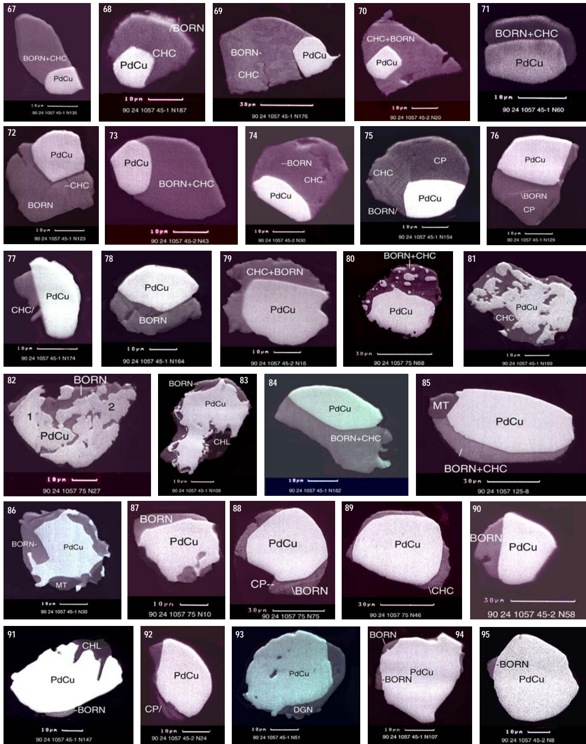
Plate 3 continued. Sulphide globules with inclusions of PdCu preserved after disintegration of the sample 90-24, 1057 (1-95); polished section, SEM-image (BIE).
