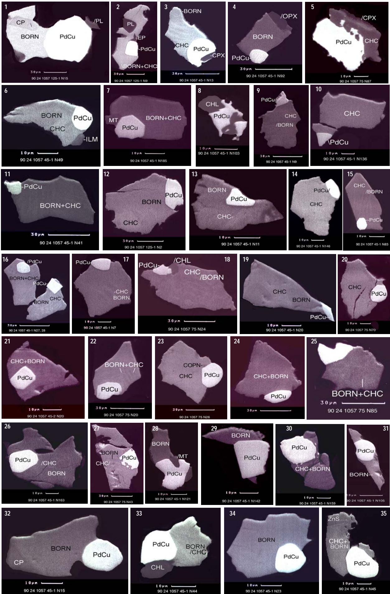
Plate 4. Sulphide globules with inclusions of the PdCu mineral phase in heavy concentrates that are partly destroyed during disintegration of the sample 90-24, 1057 (1-81); polished section, SEM-image (BIE).
