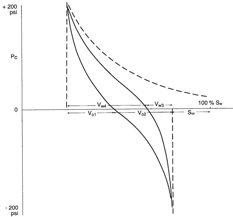
Fig. 4.2. Hysteresis loop showing the relationship between Amott's wettability and capillary pressure curves for a mixed-wet system.
