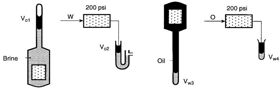
Fig. 4.1. Sketch showing the four steps of Amott's wettability test.
