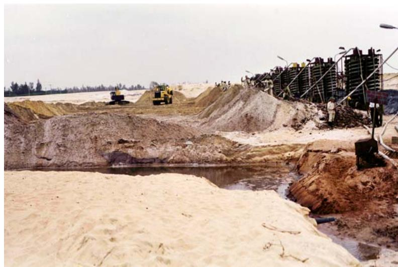
**Figure 5.** Cam Hoa # 1 open pit. The black sand layer is close to the water table.
