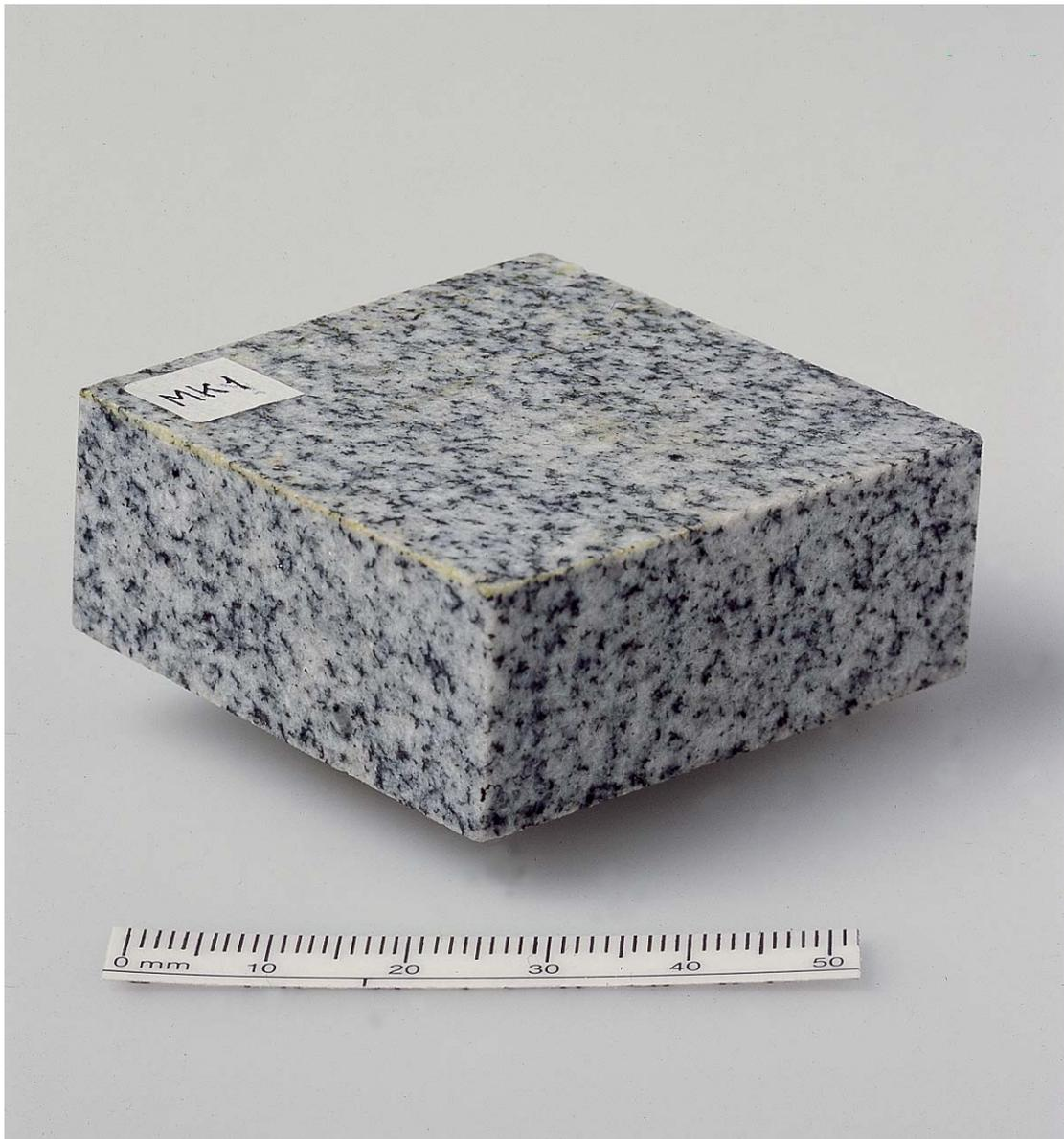
**Figure 1.** *Photograph of a cut-out hand specimen of the granite panel representing an example for Chinese granite panels. Note the only slight preferred orientation of mafic minerals in the panel.*
