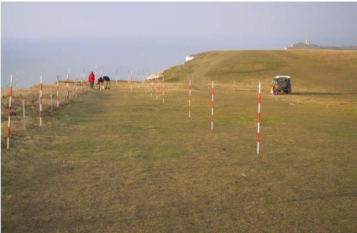
**Figure 13.** *The field above the chalk cliff at Beachy Head, where the test grid is established. Note the field team carrying out the azimuthal resistivity measurements.*
