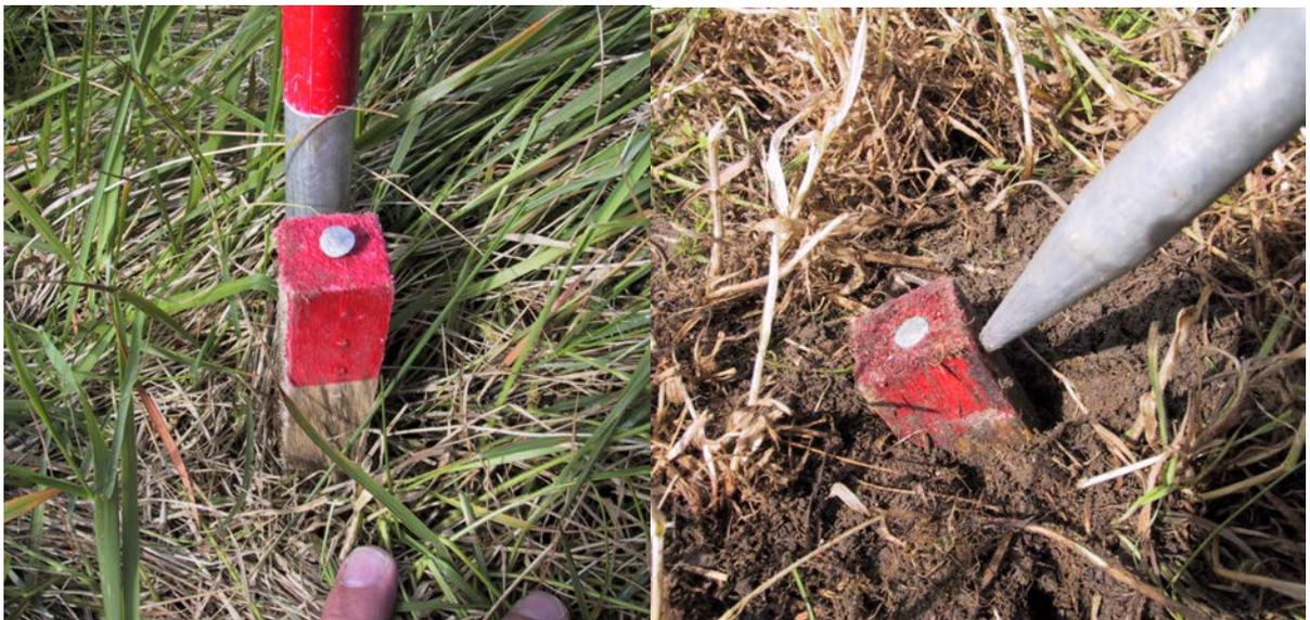
**Figure 22.** *Grid point established in the test grid consists of a wooden peg about 30 to 50 cm long (left) hammered into the chalky ground. In part of the Mesnil-Val grid the points were destroyed during the constructional work related to the establishment of the acoustic sensors (right), and these point had to be re-established subsequently.*
