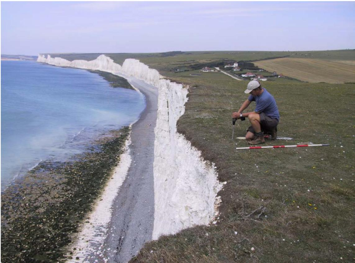
**Figure 1.** *Establishment of a grid point in the Birling Gab, Eastbourne, test site. First a drill hole was prepared for hammering a wood peg into the ground, which hampered the hammering activity to avoid cliff collapse initiated by hammering along the edge of the cliff. On top of the peg a nail marks the precise position of the point.*
