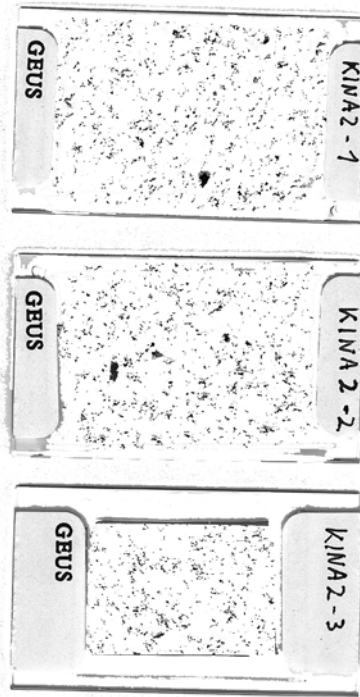
Figure 18. Scans of the 3 different thinsections made from sample Kina2. Note that there is no shape preferred orientation of biotite and that the crystals are coarse grained. For orientation of thinsections see Figure 2. Length of slides ca. 5 cm
