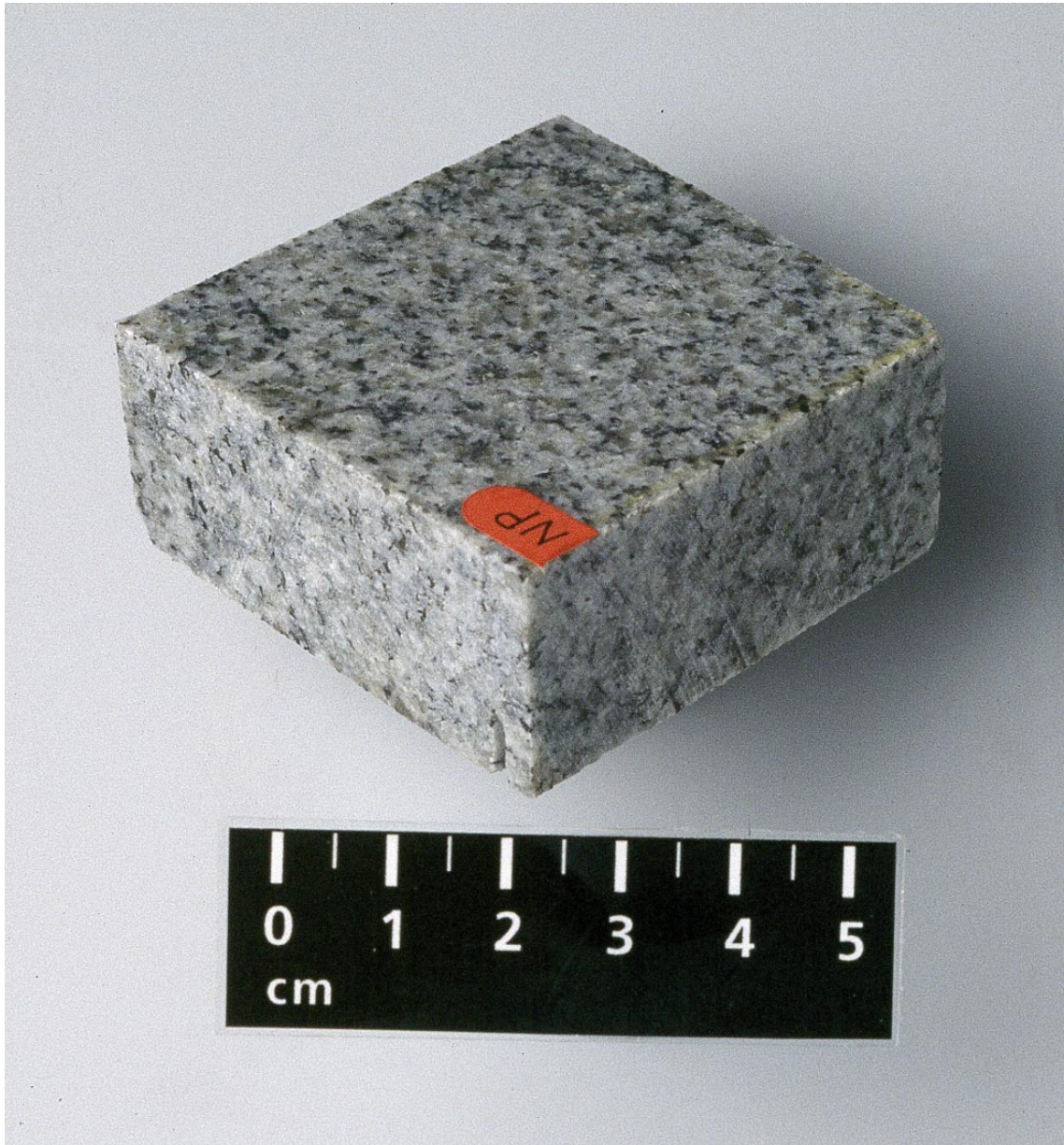
Figure 33. Cut-out handspecimen of sample NP1, granite from Nørreport Metro Station. Note there is no discolouration on the top surface and the igneous, unfoliated and lineated appearance of the rock.
