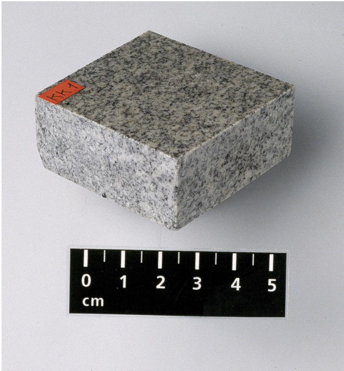
Figure 3. Cut-out hand specimen of sample Kina1, granite from Kongens Nytorv Metro Station. Note the discoloration on the top surface and the foliated and lineated appearance of the rock.
