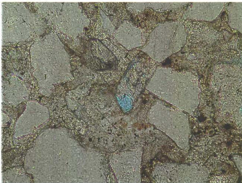
Plate 24. This detailed view shows a secondary pore, which occur in the pore occluding carbonate cement. The pore space is now partially filled by carbonate cement. Field of view 0.7 x 0.5mm, PPL.
