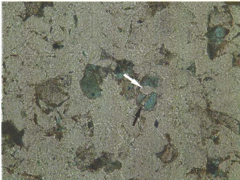
Plate 68. This detailed view shows secondary pores in the area where quartz cement occludes pores. A second quartz cement is seen growing as syntaxial crystals in a secondary pore (white arrow). Later a baryte needle has grown in the same pore (black arrow). Field of view 1.0 x 0.8mm, PPL.
