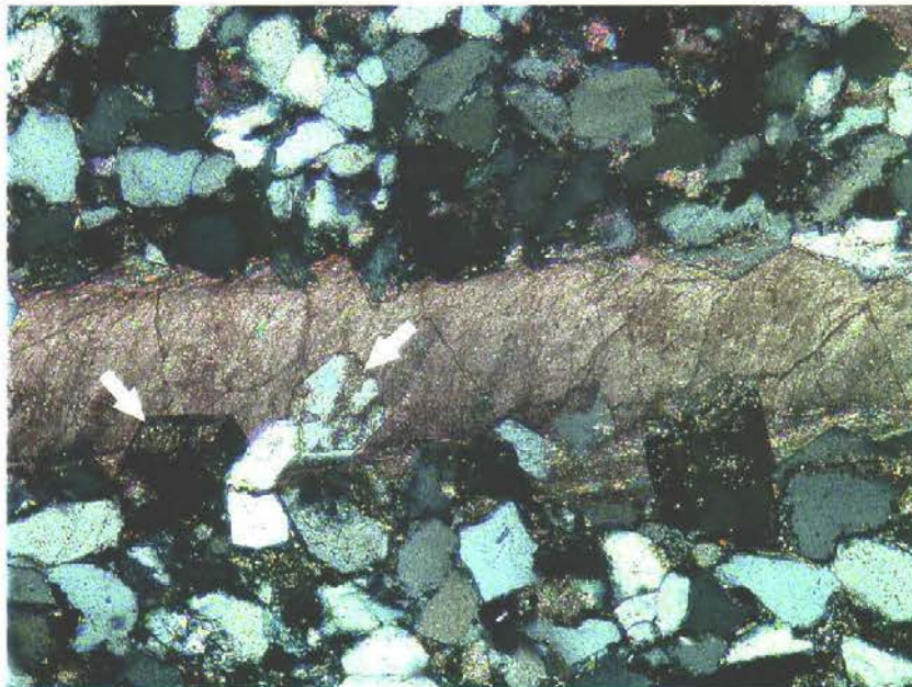
Plate 32. Syntaxial quartz has grown into a shell fragment and replaced the calcite. Note the presence of abundant calcite inclusions in the quartz crystals (arrowed). Field of view 1.1 x 0.8mm, XPL, Alizarin Red S stained.
