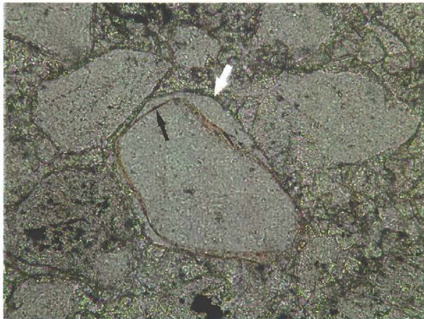
Plate 46. This detailed view shows a quartz grain displaying a conspicuous dust-rim (black arrow) and a rounded overgrowth (white arrow). The rounded nature of the overgrowth indicate that it originate from a former sedimentary cycle. Field of view 0.5 x 0.4mm, PPL.
