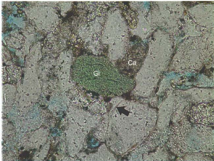
Plate 50. This view shows a weakly deformed glauconite pellet (Gl), carbonate cement (Ca) and a quartz overgrowth clearly defined by a dust-rim (arrowed). Field of view 0.6 x 0.4mm, PPL.
