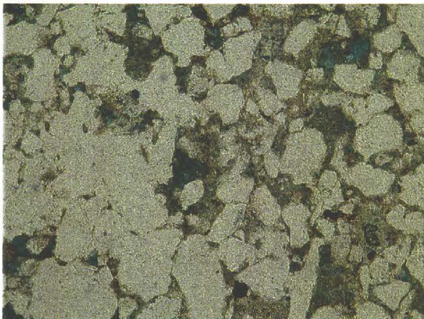
Plate 62. This view shows the reduced interconnectivity between pores due to quartz cement and detrital clay. Note that small secondary pores occur. Field of view 1.3 x 1.0mm, PPL.
