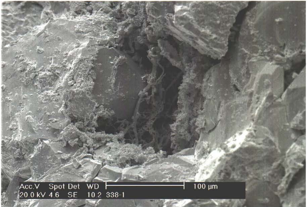
Plate 71. The photograph shows a secondary pore with a clay rim on the surfaces of former feldspar. Parts of the clay rim consist of a network of tangled illite threads (see plate 72). Note that the pore space is closely surrounded by well developed quartz cement.
