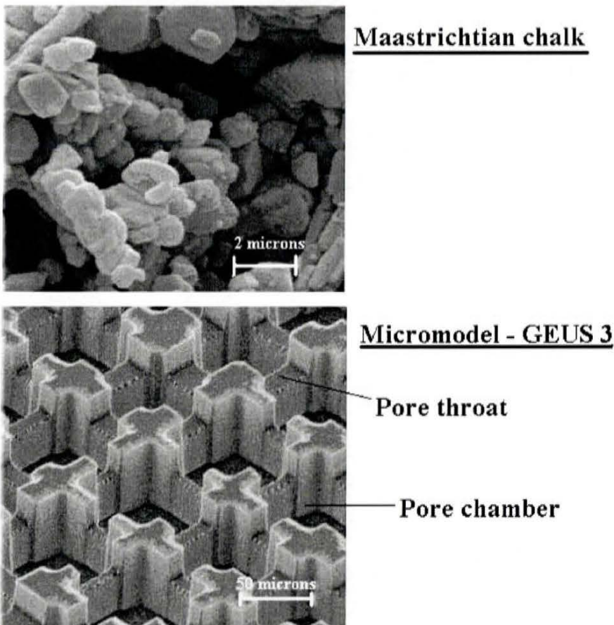
Figure 1.3. Two SEM pictures: (1) pore space of Maastrichtian chalk from the North Sea. (2) Pore space of an artificial porous network, (micromodel) etched in a silicon wafer.
