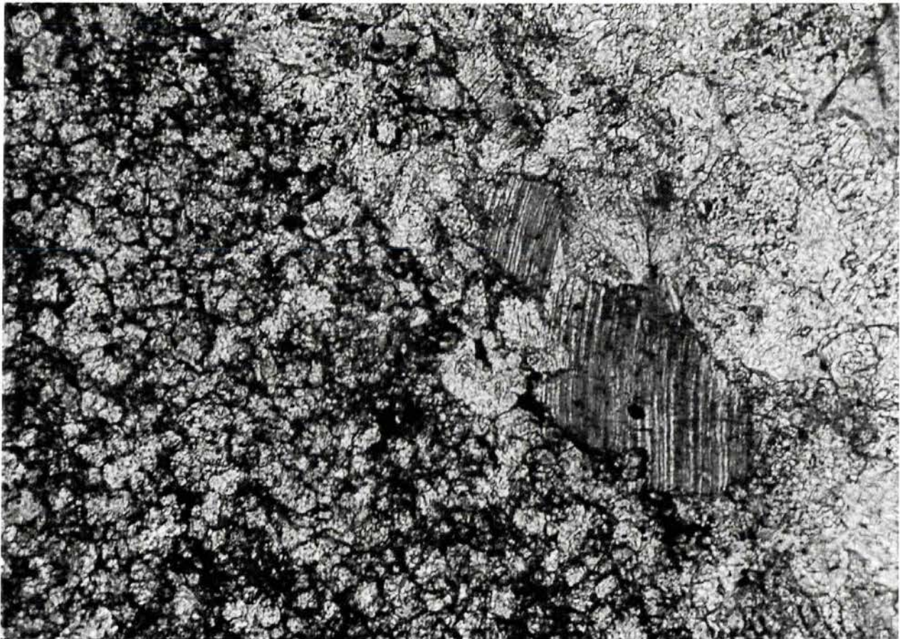
Figure 2. Thin section photomicrograph showing a stylolitic contact between a spar-filled fracture (the coarse-grained crystals to the right) and the surrounding rock matrix. The latter has been exposed to an aggrading neomorphism, perhaps contemporaneously with a similar neomorphism of the coarsely crystalline fracture spar. The presence of residuals of the stylolite seam inside some of the sparry crystals indicate that a phase of recrystallization post-dates the phase of chemical compaction. Width of view is 0.9 mm (Sample 1A-1).
