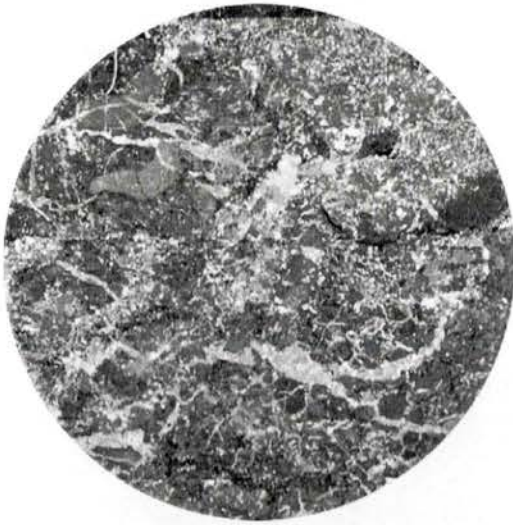
Figure 17: A thin section of the marbled limestone of sample 2-1, being rich in fine almost hairline-like fractures and irregular vein-like patches of sparry calcite. The section is about 25 mm in diameter.
