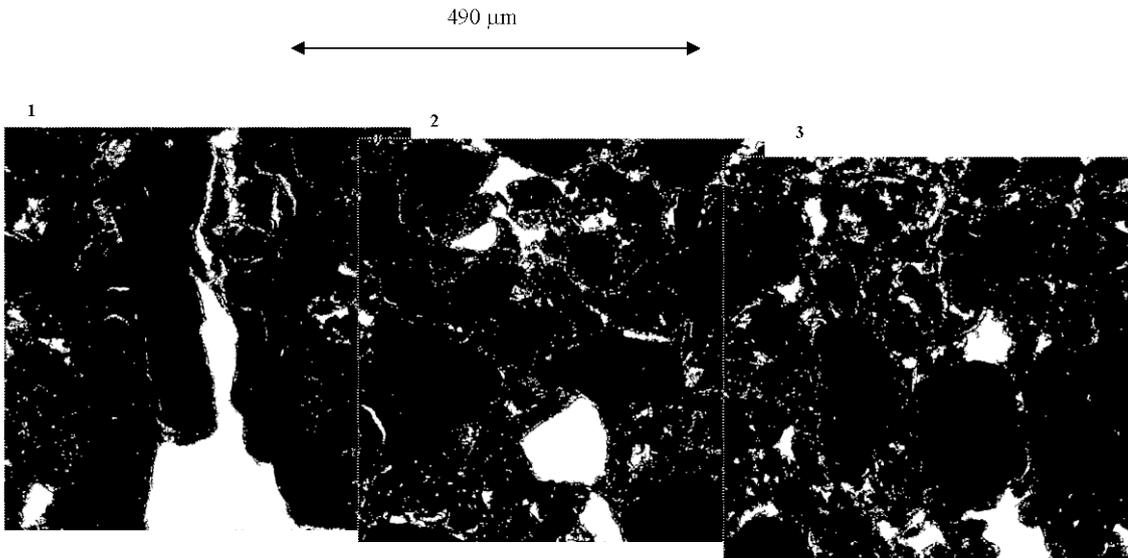
Figure 27. Binary-images (200x) of “the fracture zone” in sample 10A.
