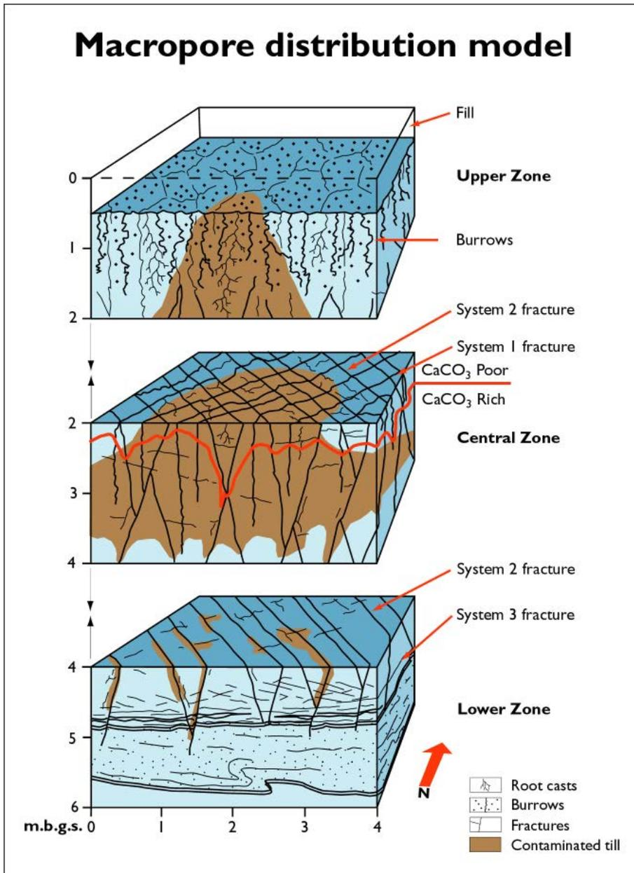
**Figure 2. Macropore distribution model near Pit 2 and 3. The distribution of LNAPL is marked and since the system 2 fractures seems to be the dominating fractures most of the intact samples were collected from this fracture system.**
