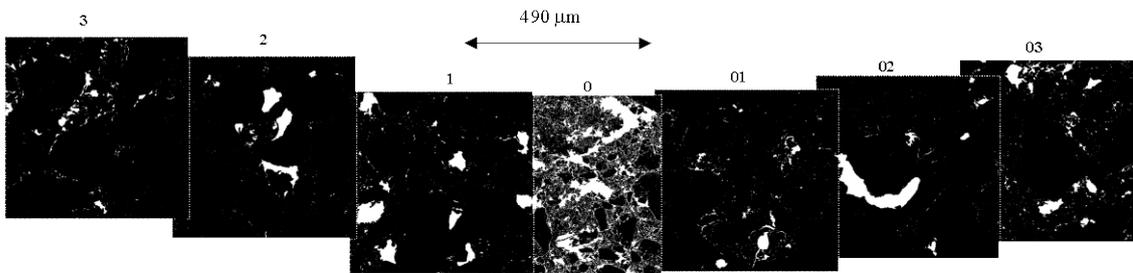
Figure 9. Binary images (200x) of “the fracture zone” in sample 4T.
