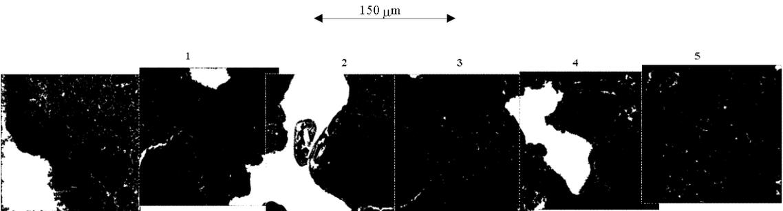
Figure 20. Binary images (800x) of “the fracture zone” in sample 7.2A.
