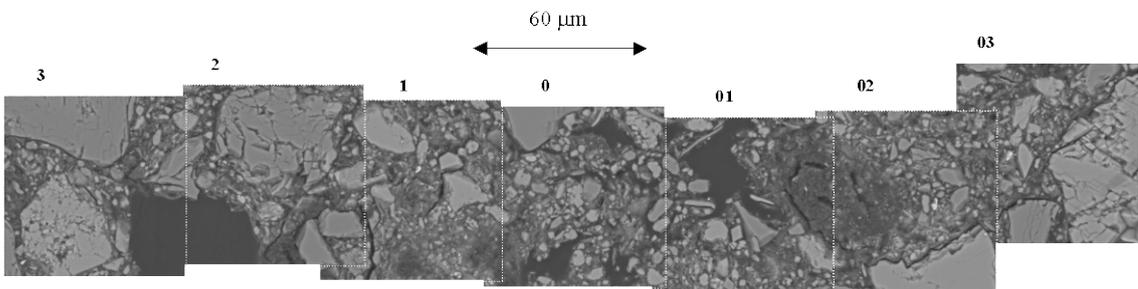
Figure 14. Vantage SEM-images (1600x) of “the fracture zone” in sample 4T.
