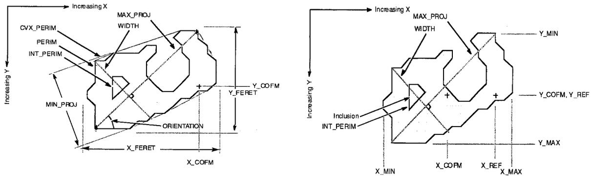
**Figure 3. Visualisation of: (a) Basic particle parameters and (b) Basic frame parameters.**
