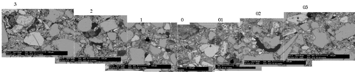
Figure 7. SEM-images (200x) of “the fracture zone” in sample 4T.
