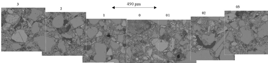
Figure 8. Vantage SEM-images (200x) of “the fracture zone” in sample 4T.
