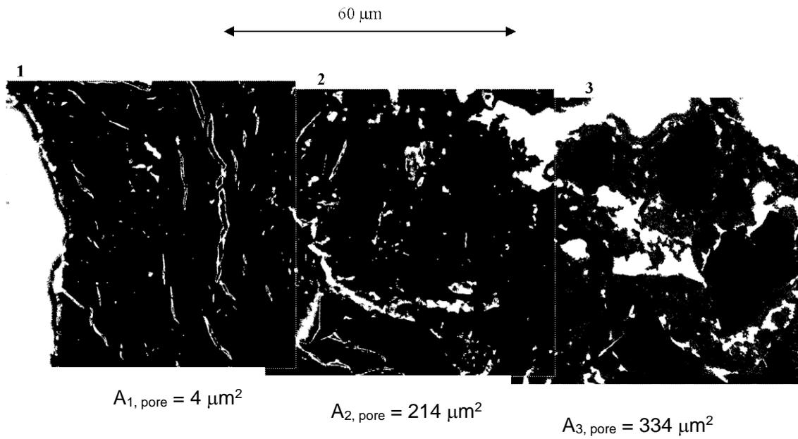
**Figure 30. Binary images (1600x) of “the fracture zone” in sample 10A. Below the images the natural pore area A of each images are noted.**
