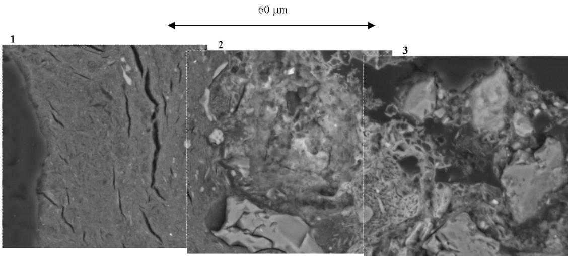
Figure 29. Vantage SEM-images (1600x) of “the fracture zone” in sample 10A.
