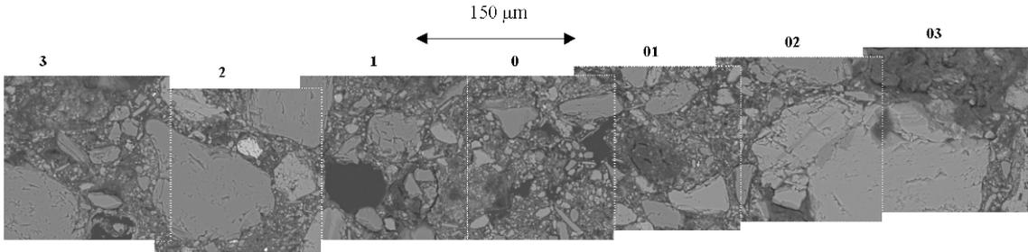
Figure 11. Vantage SEM-images (800x) of “the fracture zone” in sample 4T.
