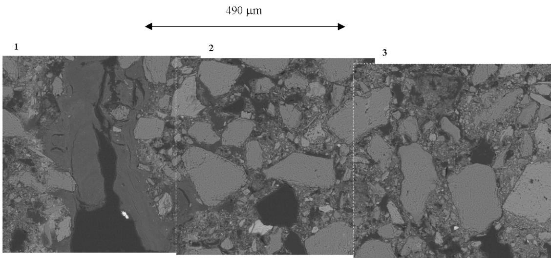
Figure 26. Vantage SEM-images (200x) of “the fracture zone” in sample 10A.
