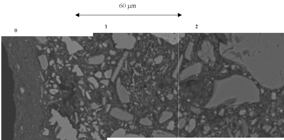
**Figure 22. Vantage SEM-images (1600x) of “the fracture zone” in sample 7.2.**
