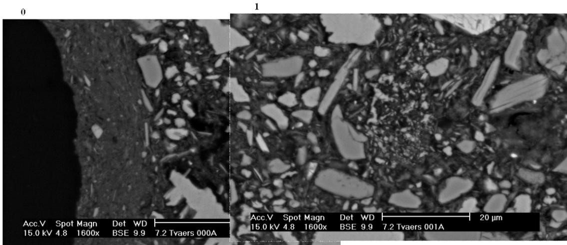
**Figure 21. SEM-images (1600x) of “the fracture zone” in sample 7.2A.**
