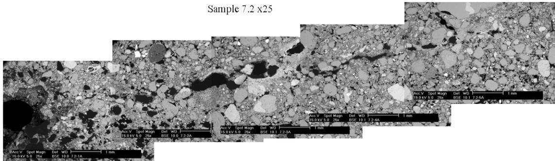
**Figure 5. SEM-images of fracture in sample 7.2A.**
