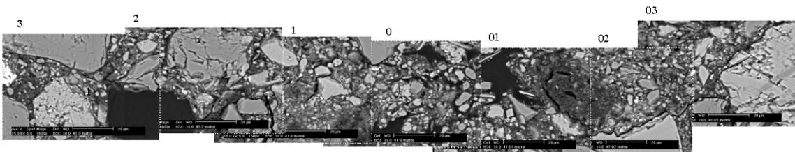
Figure 13. SEM-images (1600x) of “the fracture zone” in sample 4T.
