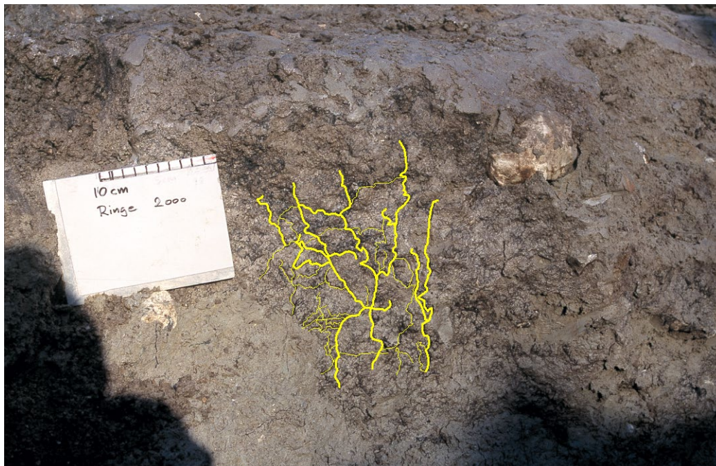
Figure 5.2 fracture surface with contamination distributed in channels.
