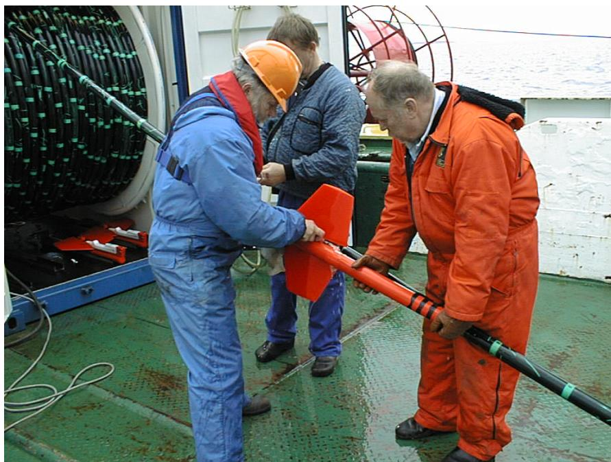
Fig. 27: Deployment of streamer – installation of bird (depth controlling device)
