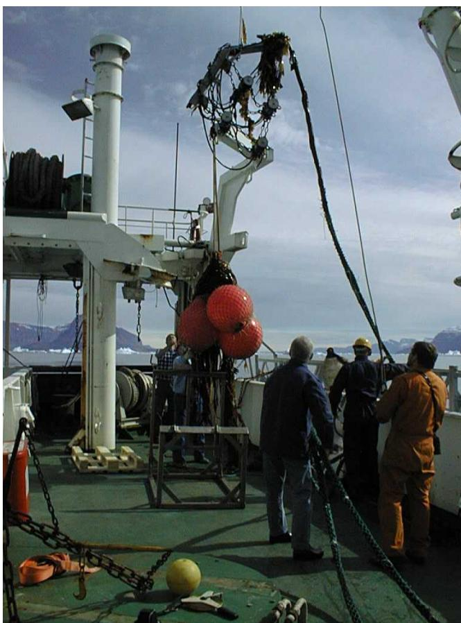
Fig. 29: Deployment of airgun array (4 x 40 cu. inch sleeve guns)
