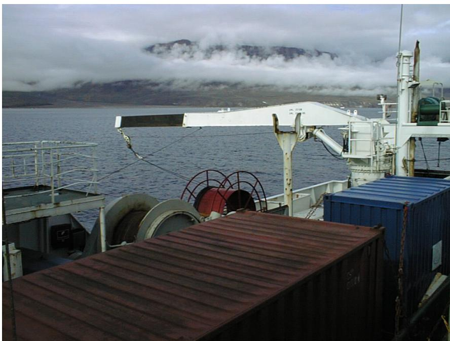
Fig. 35: Modified towing arrangement for the magnetometer sensor
