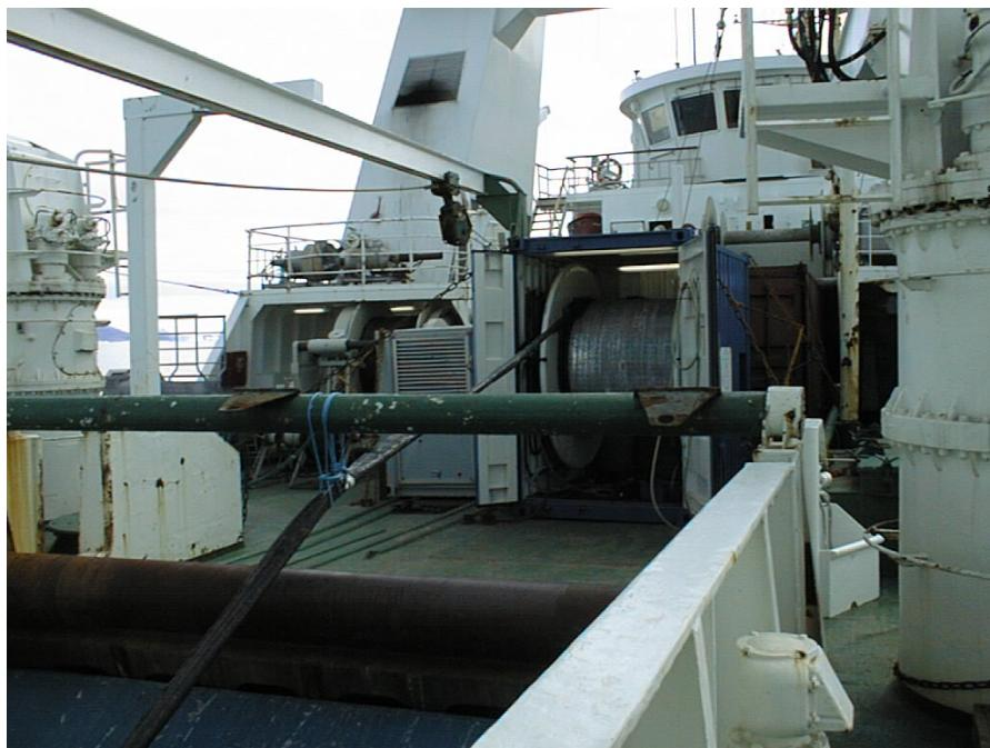
Fig. 26: Containerised streamer reel (Aarhus University) on the back deck of H/S Dana
