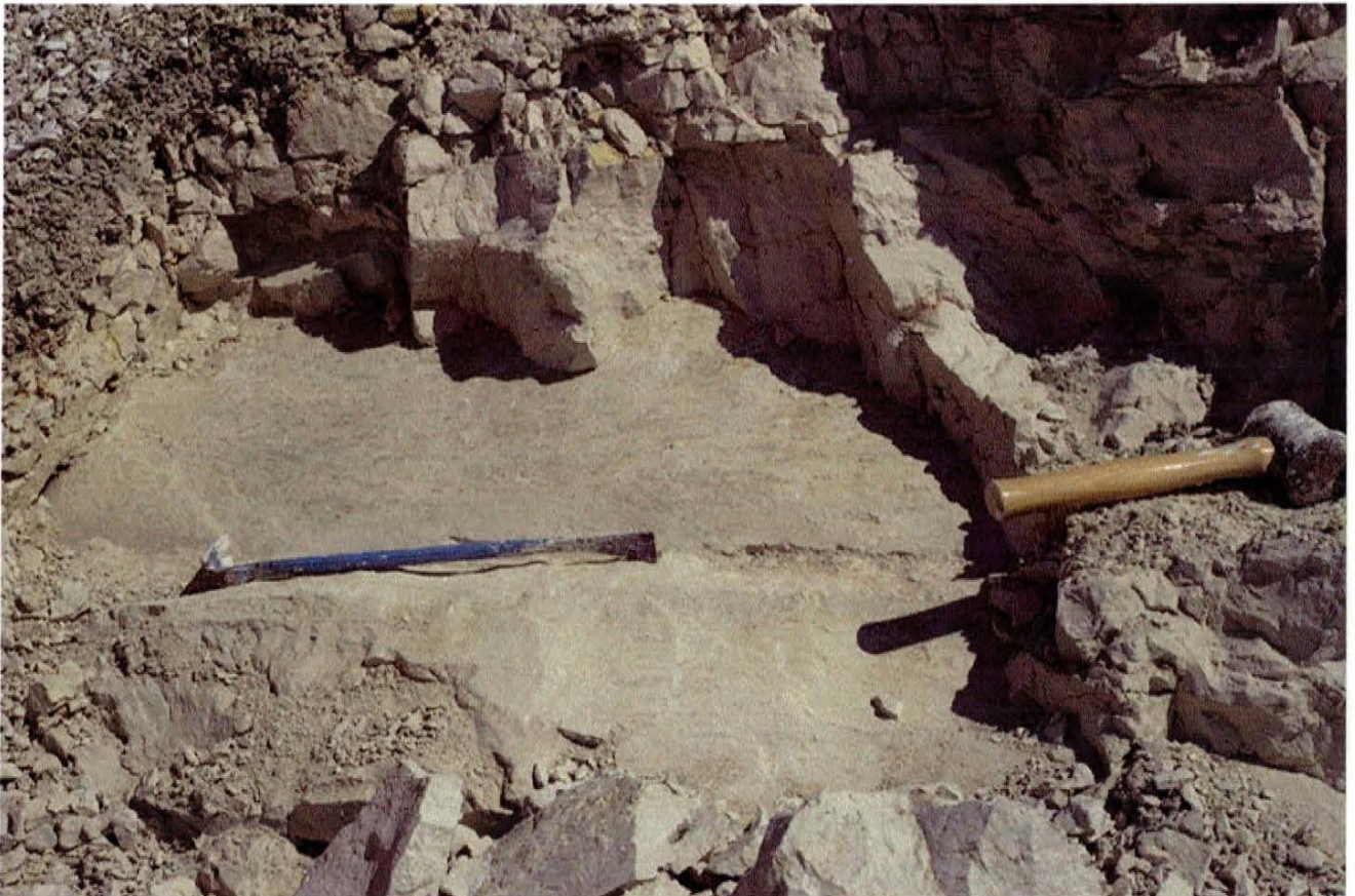
Figure 16. Gentle dipping strike-slip fractures. A) Fracture along strike direction. B) Excavated surface.
