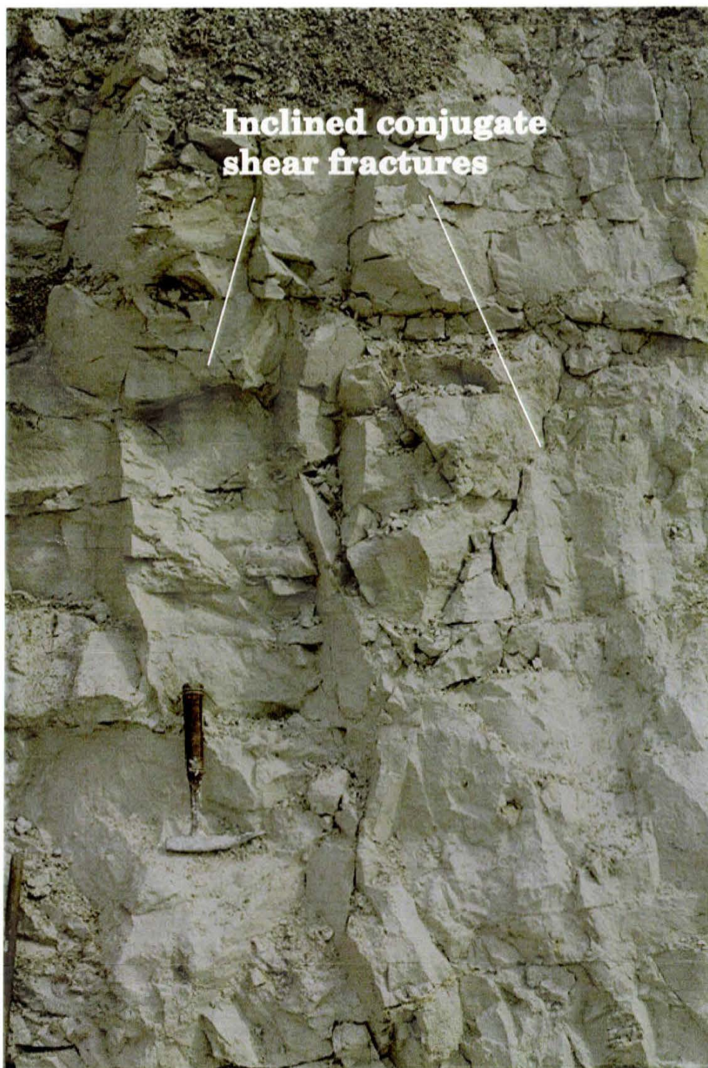
Figure 12. Example of a conjugate set of inclined shear fractures.
