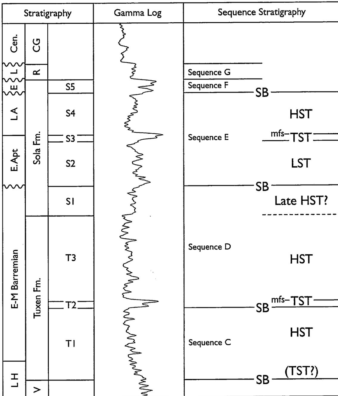
Figure 3. Sequence stratigraphic subdivision of the Tuxen and Sola Formations in the North Jens-1 well (From Ineson, 1994).
