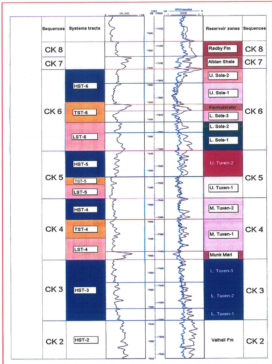
Figure 7: Proposed zonation of the Barremian to Albian section in the North Jens-1 well correlated with recent established sequence stratigraphy and determined systems tracts. The zonation corresponds only to some degree with the systems tracts due to the lithological variation within the various systems tracts.
