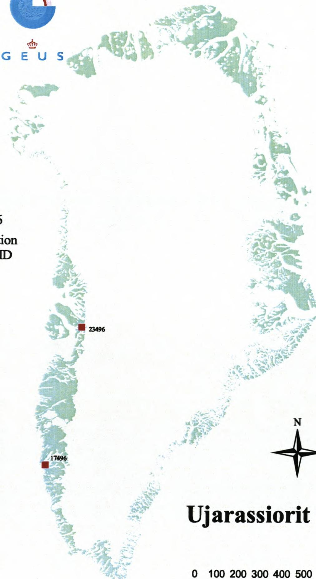
Fig.6. Location of samples with anomalously high Mo and/or W content
