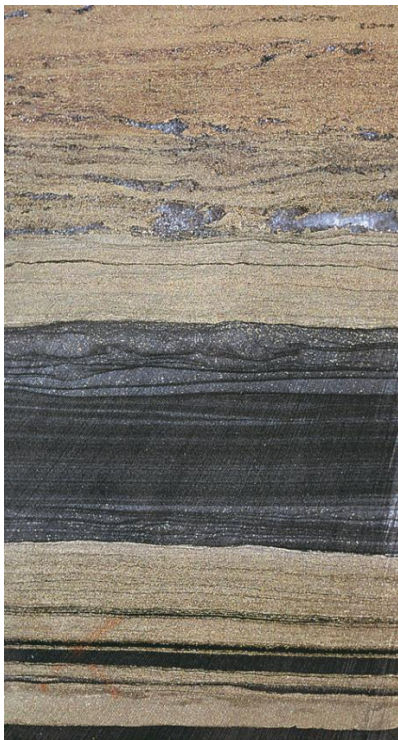
Figure 19. Fine-grained laminated sulphides in black mudstone. The sulphide laminae consist of framboidal pyrite in a matrix of sphalerite and carbonate. Zn-content in the upper sulphide layer is 25-30% and in the lower layer 1-3%. Platinova drill-core CF-15, 3.6 cm across. From Kragh (1996).
