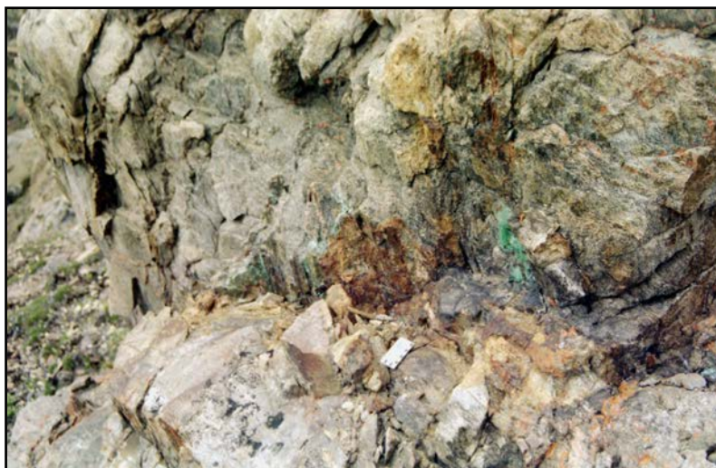
Figure 28. Close-up of the gold bearing horizon in the shear zone with malachite staining (just above the white scale card, 5 cm wide).
