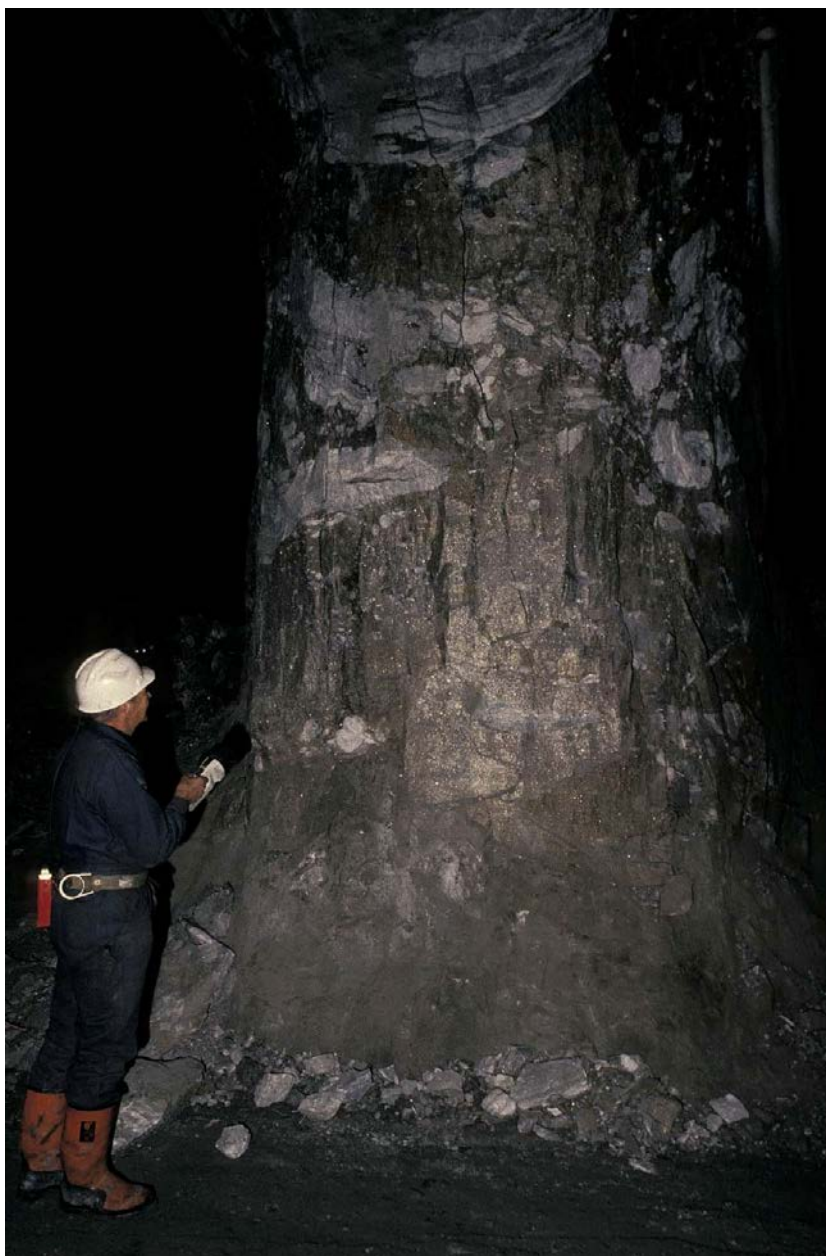
Figure 81. "Buck shot ore" (massive sulphide) with marble rafts left in pillar in the underground mine area of the 'Black Angel' mine.
