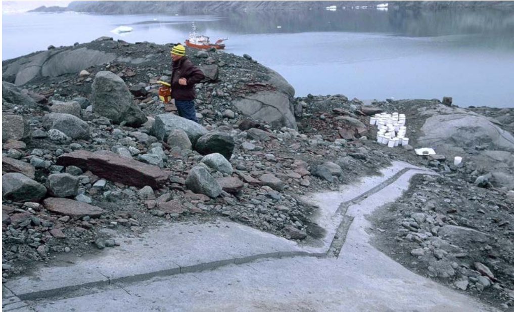
Figure 53. Channel sampling at Skaergaard.
