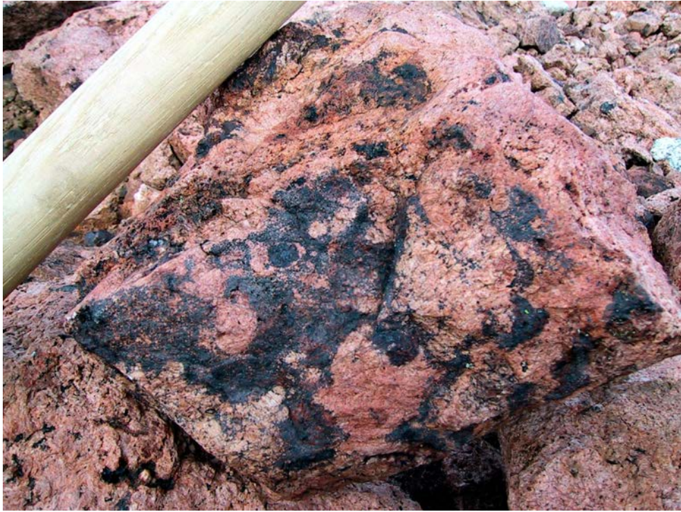
Figure 67. Close up of the pyrochlore mineralisation in syenite of the Motzfeldt Sø formation .
