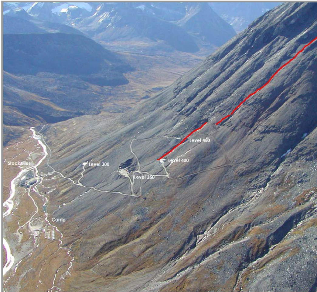
Figure 46. Kirkespirdalen with Nalunaq gold mine. Red line outlines the gold-bearing Main Quartz Vein.
