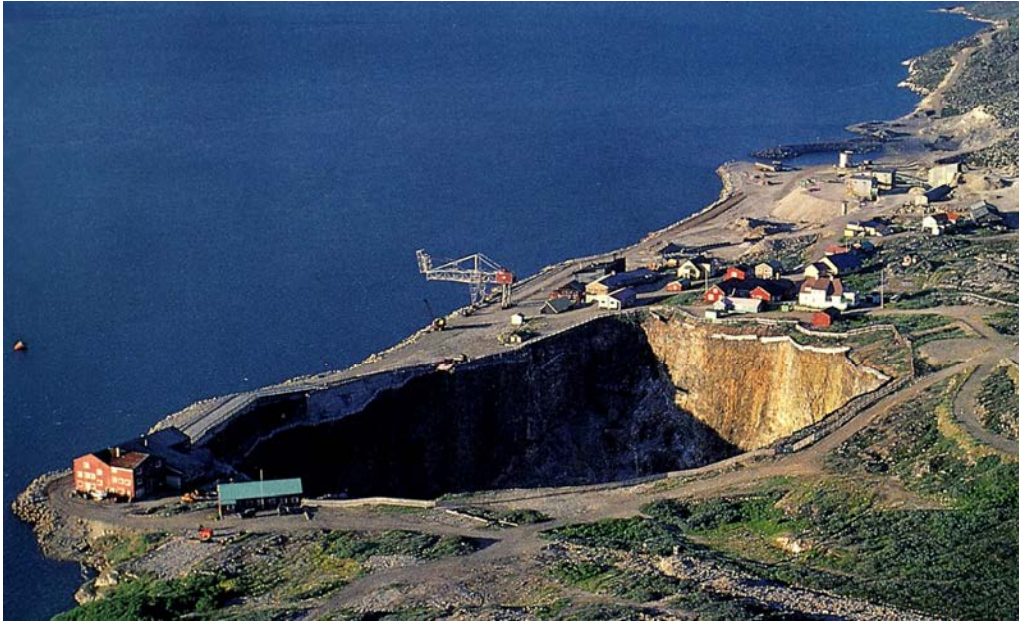
Figure 64. Aerial view of the abandoned cryolite mine in Ivittuut, 1987. The open pit has the shape of the now exploited cryolite body.
