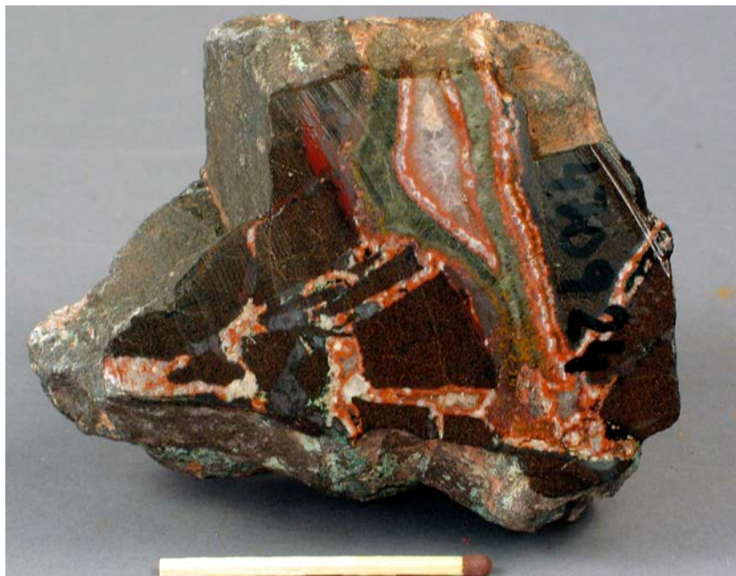
Figure 8. Cut surface of volcanic scree block with hematite-chalcocite-bearing quartz-calcite veins and 1.1% Cu, 8.9% Fe. West side of Parish Gletscher (470924). Match is 5 cm; photo: Jakob Lautrup.
