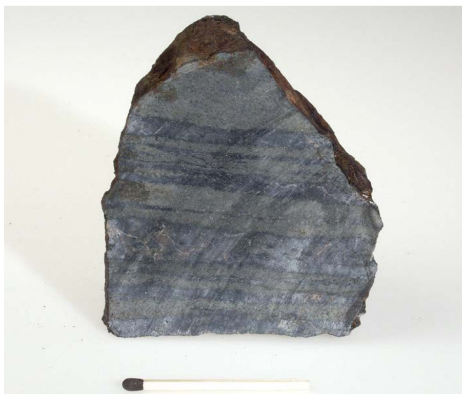
Figure 4. Cut surface of pyrrhotite-magnetite bearing BIF with 16% Fe. Thule mixed-gneiss complex, Noorupaluk (470952). Match is 5 cm. Photo: Jakob Lautrup.
