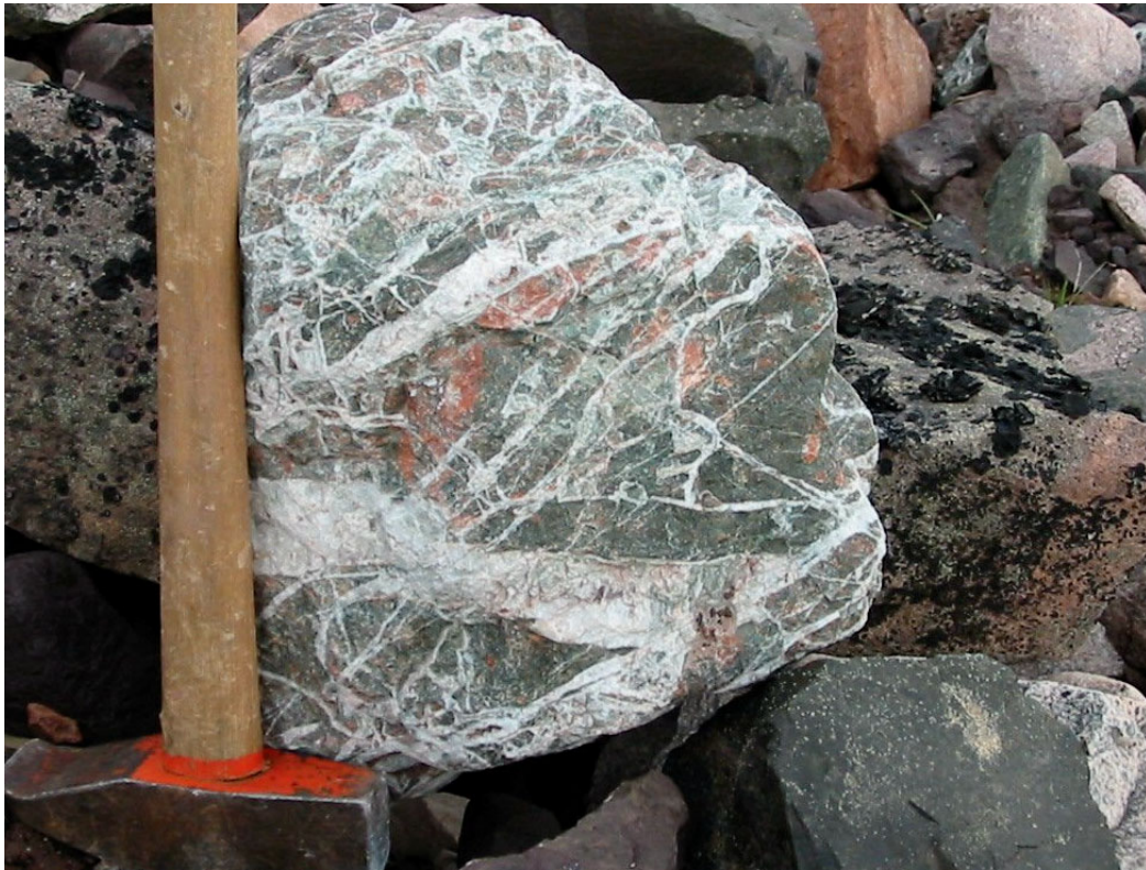
Figure 13. Moraine block from western Parish Gletscher of silicified volcanic rocks with blebs of chalcopyrite-pyrrhotite and 0.6% Cu, 0.9% Fe and 0.7% Ba (470925).
