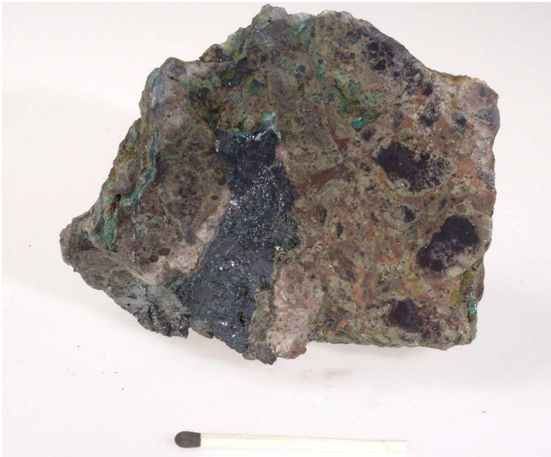
Figure 11. Cut surface of hematite-chalcocite-bearing volcanic float with 1.7% Cu, 21.9% Fe (470939). From locality shown on Figure 10. Match is 5 cm; photo: Jakob Lautrup.
