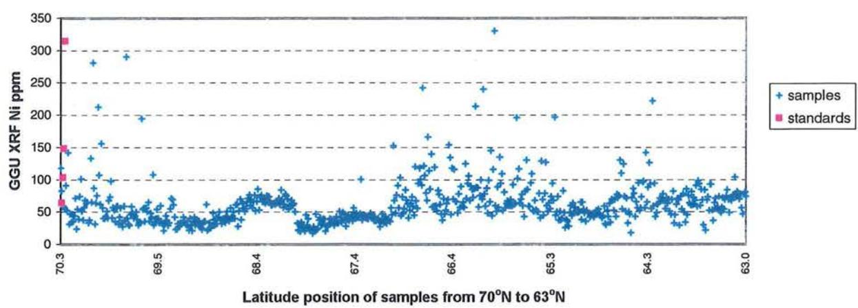
**Figure 5.** Range of Ni concentrations measured in standards and in samples within a longitudinal section through the atlas region. Laboratory: GGU (Geological Survey of Greenland). Method: XRF (X-ray Fluorescence Spectrometry).
