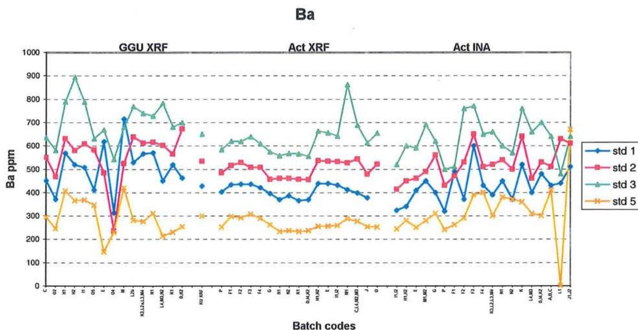
**Figure 6a-m.** Variability of analytical results from various sources as monitored by standards. Laboratories: GGU (Geological Survey of Greenland); Act (Activation Laboratories Ltd.); KU (Geological Institute, University of Copenhagen). Methods: XRF (X-ray Fluorescence Spectrometry); INA (Instrumental Neutron Activation); ICP (Inductively coupled Plasma Emission Spectrometry).
