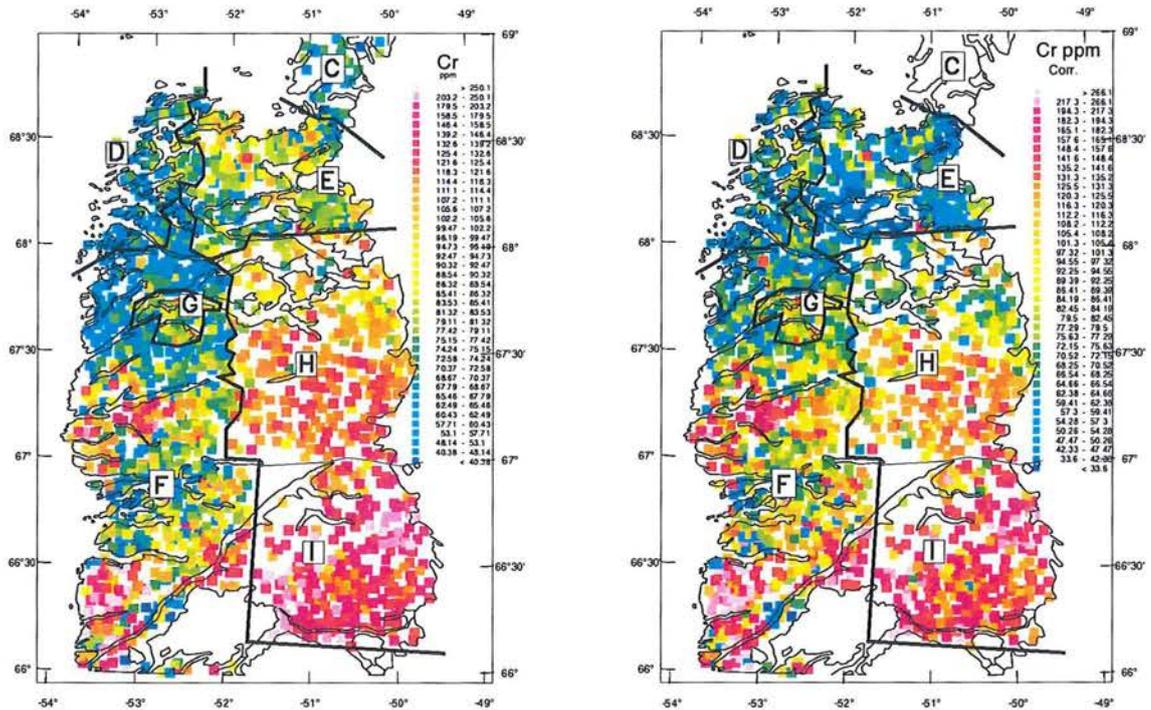
**Figure 20.** The effect of calibration. Geochemical maps of Cr by Act XRF for a part of the atlas area. The map of uncalibrated data (left) shows the effect of the analytical bias influencing the batches from the areas E, H and I in the range around 200 ppm and below, see Fig. 14b. The false geochemical boundaries coinciding with the boundaries between surveys (heavy lines) have been eliminated in the map of calibrated data (right).
