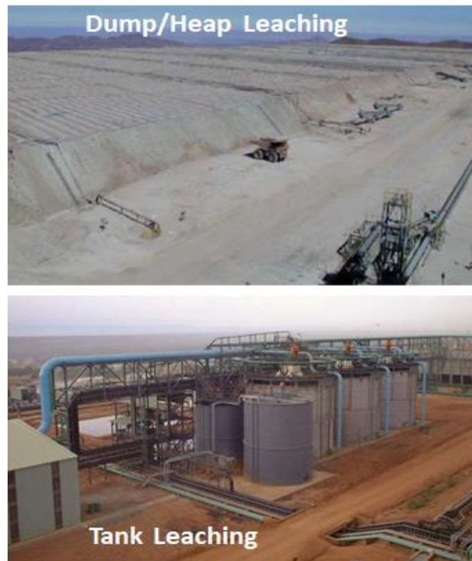
Figure 2. Dump/heap and tank leaching
