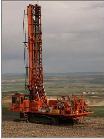
Fig. 2 Rotary drill rig
