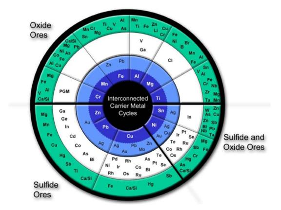
Figure 1: The "Metal Wheel" showing the relation between carrier metals (dark blue), co-elements that have their own production infrastructure (light blue), co-elements that have no, or limited own production
