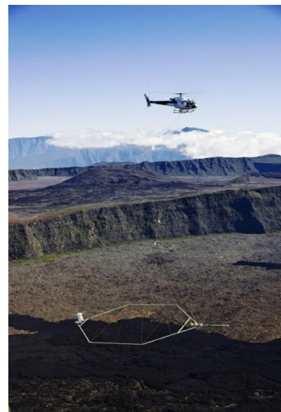
Image 1 - Airborne geophysical survey (copyright BRGM, R. Carayol)
