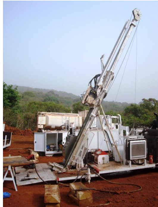
Image 2 - Core drilling exploration campaign (copyright BRGM, G. Bertrand)
